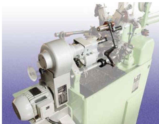
Drilling and threading attachment (BGSE) with swing stop.
